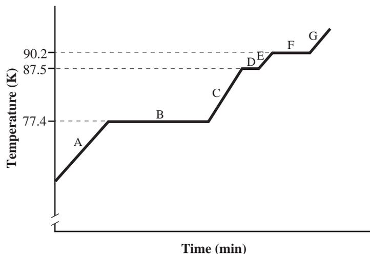
Through careful distillation, the three main components of liquid air can be separated. Their respective boiling points are
